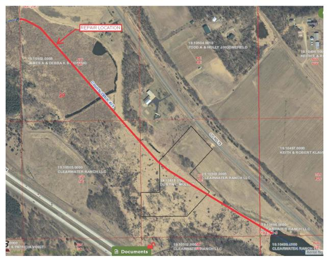
3. Restore the repair location to form a 4 foot bottom with a 2:1 side slope.
